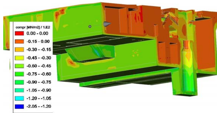
Figure 19: Contour-plot for compressive stress generated by restrained swelling at present time - red represents low compressions, green means higher stress state
