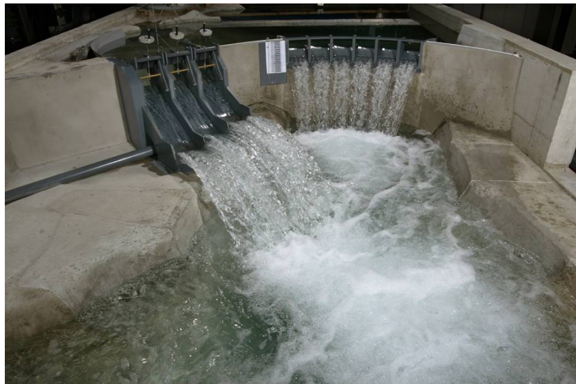
Figure 2: Shahryar dam model in the laboratory
